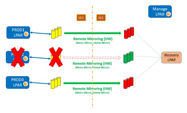
3/ The FLSTRDRP command makes an inventory of the disks contained in the consistency group specified in the definition, and maps them to the recovery host.
