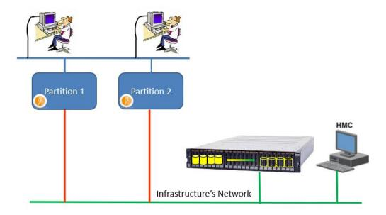
The Proxy module allows the separation of networks to be re-established by inserting an additional IBM i partition, which will be referred to as the "Proxy partition" in the following.
